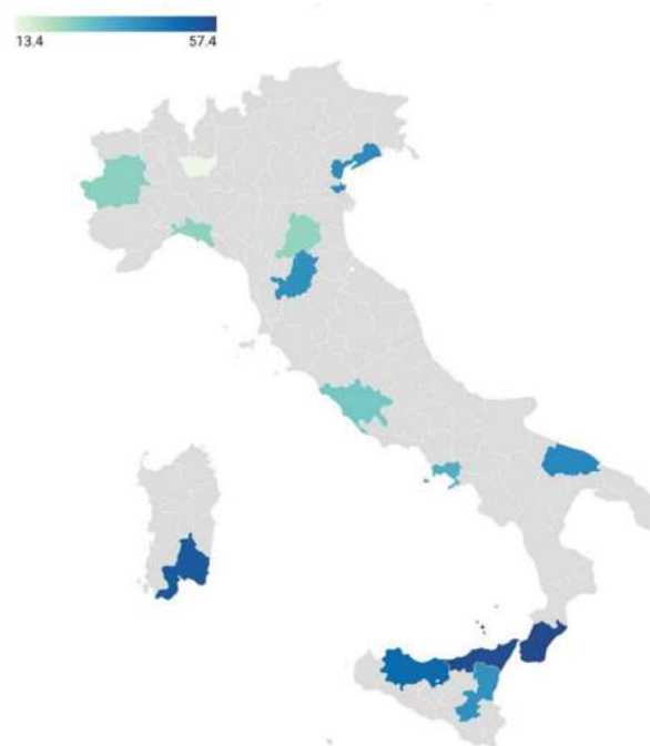
Figure 1: Volume of total water losses on the water introduced into the network (2023).
